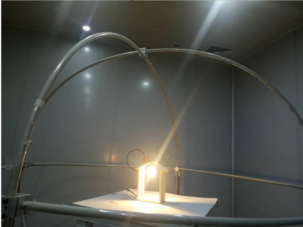
Radiated Electromagnetic Disturbances Test Setup
