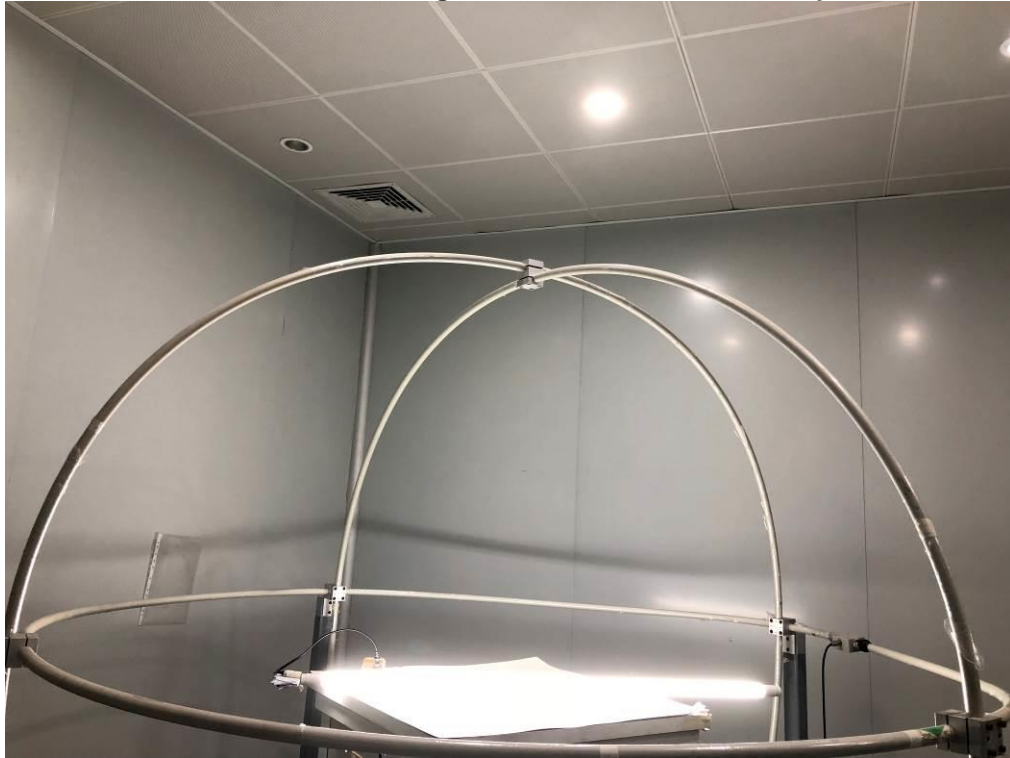
Radiated Electromagnetic Disturbances Test Setup
