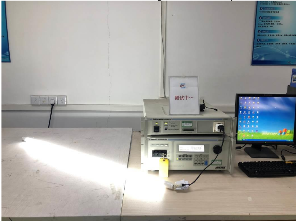
Current Harmonics /Voltage Flicker Test Setup
