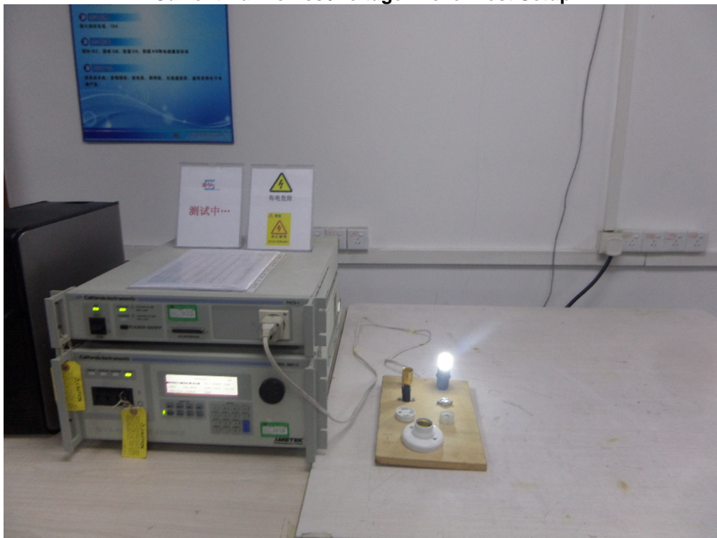
Current Harmonics /Voltage Flicker Test Setup
