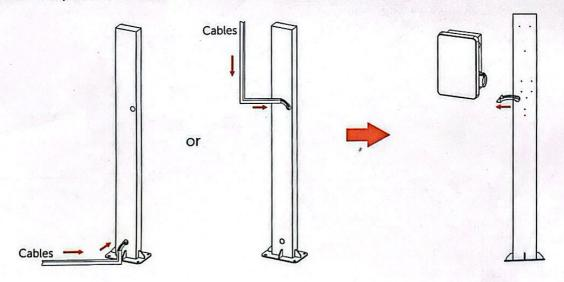
Step 6: Fix the back bracket of the EV-Charger, the holster and the cable hook on the pedestal with the screws from the accessory bag of the pedestal instead of the ones of the EV-Charger. For the installation of the EV-Charger, please refer to the corresponding manual or installation guide.
