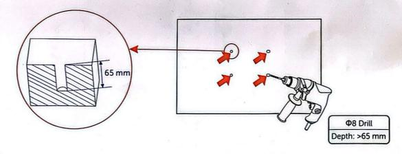
Step 3: Find the M6x80 bolts and disassemble as following. Then insert the expansion bolts with tapping screws into the drilled holes and secure the bolts with a mallet.
