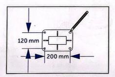
Step 2: Remove the pedestal and drill holes at the marked positions using a  $\Phi 8$  drill with a depth of at least 65 mm.
