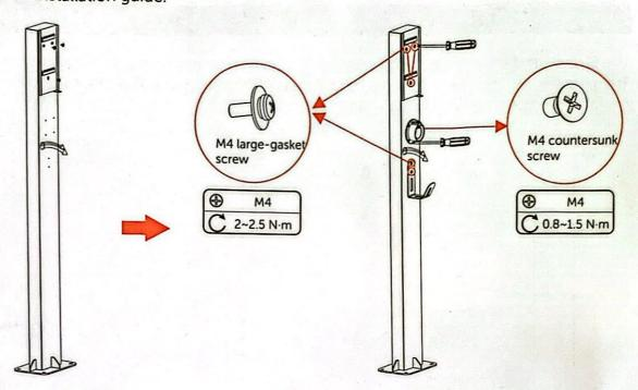
Step 7: Once the installation is completed, plug the connector to the holster and hang the cables on the cable hook.
